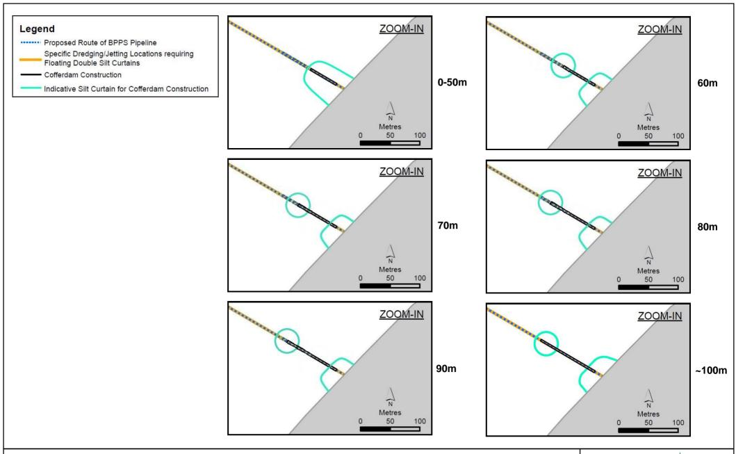
Silt Curtain Arrangement during Construction of the Cofferdam for BPPS Pipeline
