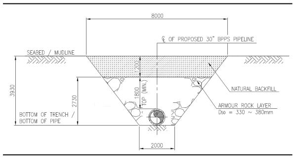
Figure 3.6 Trench Design (Type F)
