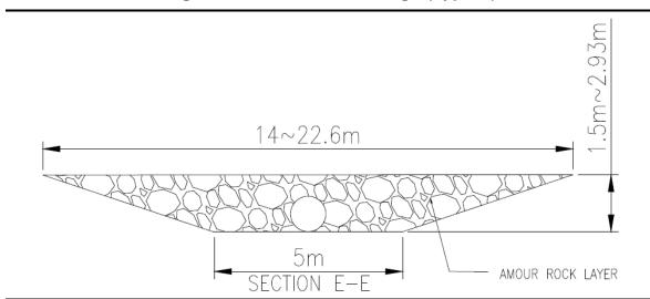
Figure 3.2 Trench Design (Type B)
