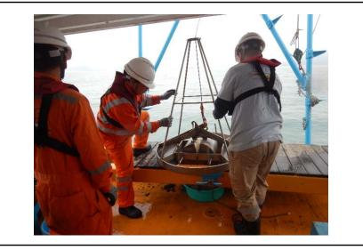
a) Sediment samples were collected using a modified Van Veen grab sampler.
