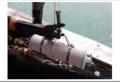
a) A Van Dorn Bottle Sampler was used to collect seawater sample.
