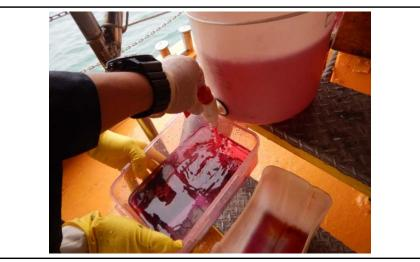
d) The materials remaining on the sieve screens were preserved using a 5% solution of borax-buffered formalin containing Rose Bengal in seawater
