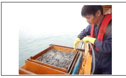
c) The sediment sample was sieved on site using a sieve stack.
