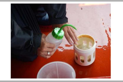
d) Zooplankton samples were filtered and fixed in 4% boraxbuffered formalin.
