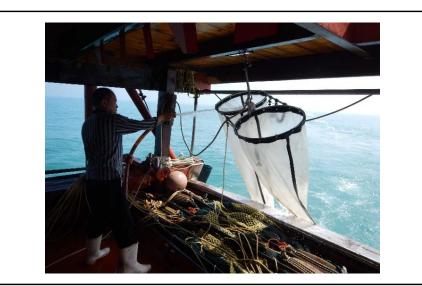
c) Plankton nets were washed after deployment at each location.
